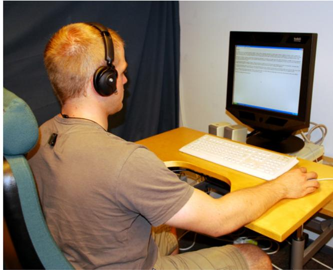
Figure 2: A test user wearing the sensors. The headset is a one-channel EEG device, the eye-tracker is integrated in the desktop monitor, and the accelerometer can be seen attached to the nape of the user. A heart rate belt is under the shirt.
